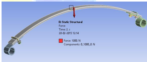
Fig.4: 1000 N Force Applied On Spring
