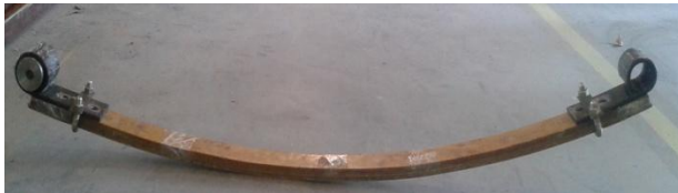
Fig.7: Final output of composite Leaf spring with steel eye.
